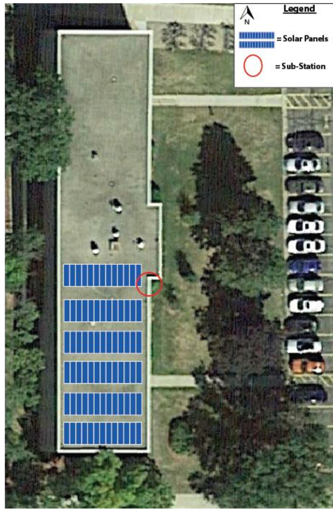
Figure 3: Proposed siting for 100 kW P.V. system on Hyer Hall
