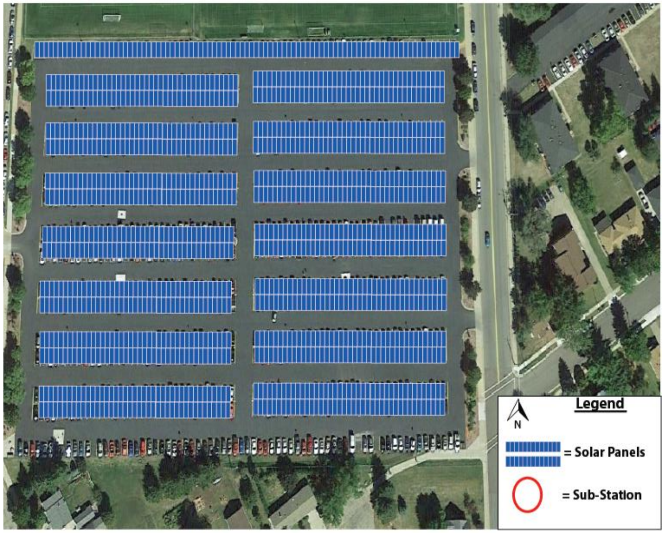
Figure 5: Proposed siting for 2417 kW P.V. system on Lot Q
