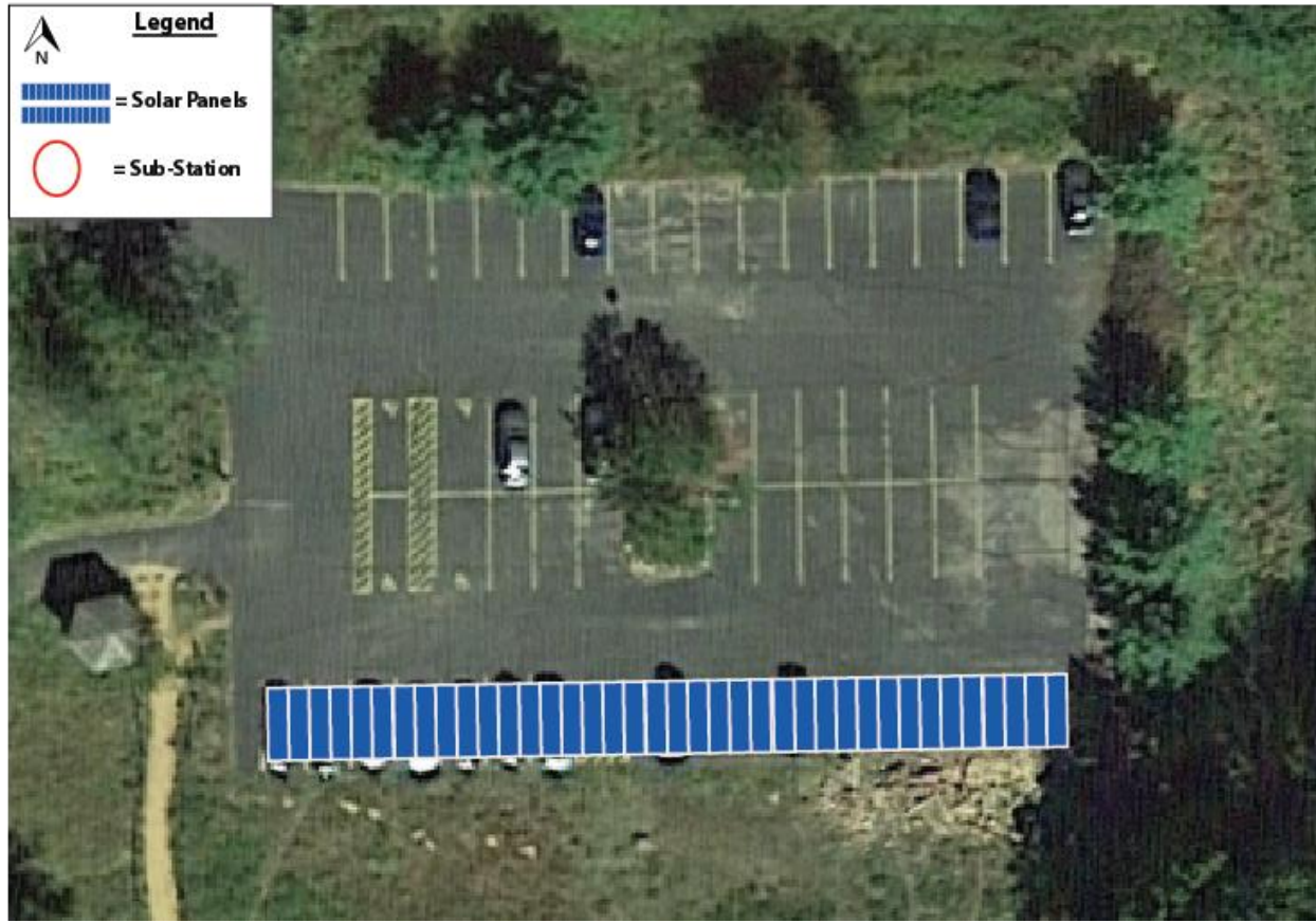
Figure 4: Proposed siting for 55 kW P.V. system on Schmeekle Visitor Center Parking Lot
